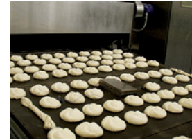
Wires from an oven profiler are inserted into Kaiser rolls, which are located on the left and right sides of the conveyor. The oven profiler monitors temperatures on both sides of the oven.
