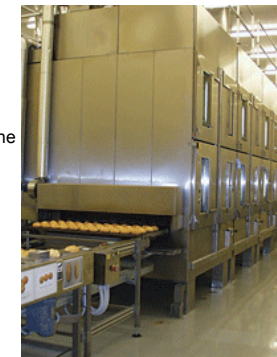
By using profilers in this serpentine oven, a Midwest bakery has reduced its baking time for Kaiser rolls and significantly increased capacity.
